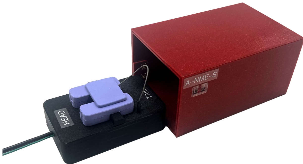
Figure 3: Neonatal mouse system setup with faraday cage.
