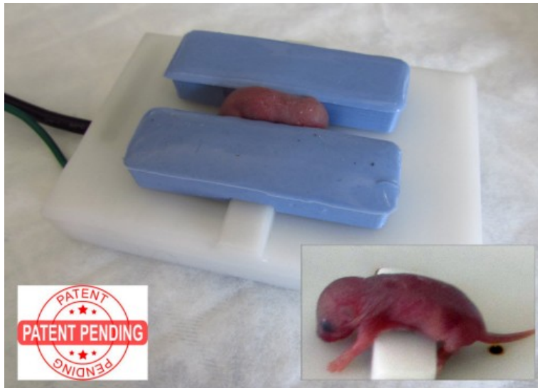
Figure 2: Neonatal Mouse setup with right and left silicone bumpers.
