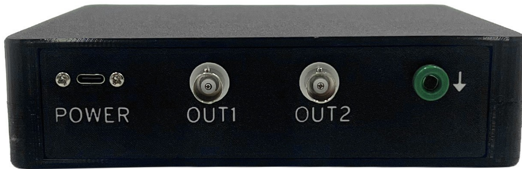
Figure 4: Back Panel USB-C Power Input, Channel 1 BNC Analog Output (OUT1), Channel 2 BNC Analog Output (OUT2), Optional Ground Port
