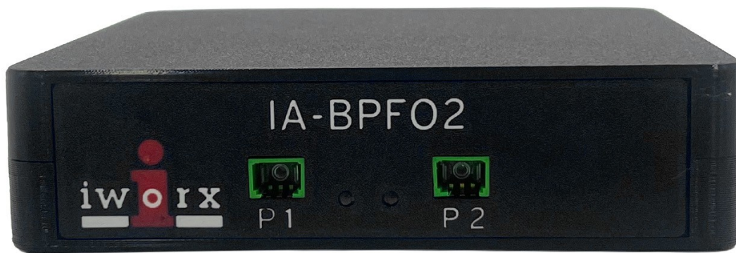
Figure 3: Front Panel Channel 1 input (P1) and Channel 2 input (P2)
