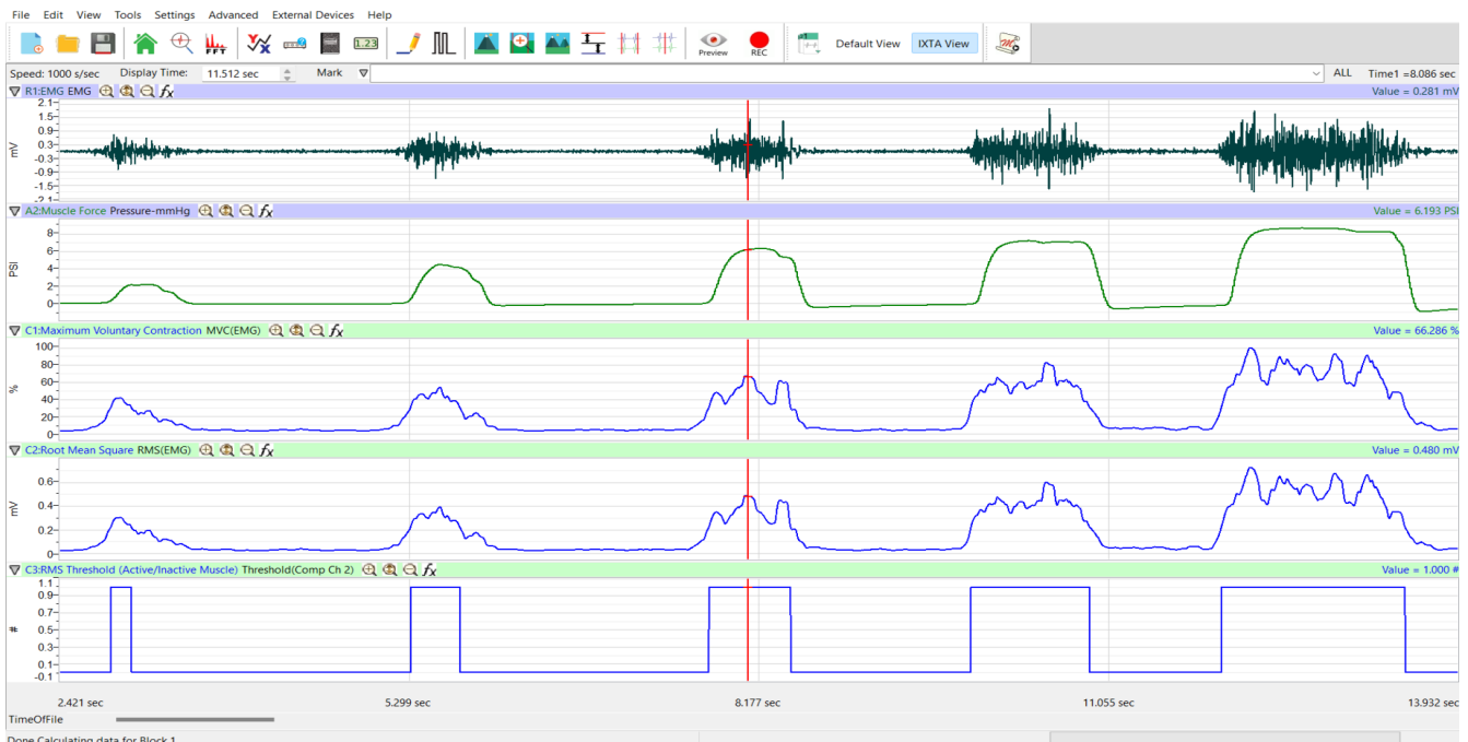
Figure: Sample EMG Recording (Channel 1 – Dark Green) and Muscle Force (Channel 2 – Light Green). Computed channels off of the EMG channel are shown in Blue, consecutively: MVC, RMS, Threshold.
