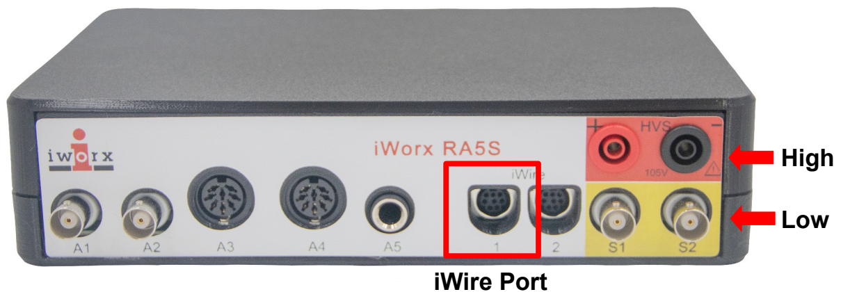
Figure 2: Front view of the IX-RA5S. The RA5S has both low voltage and high voltage stimulators.
