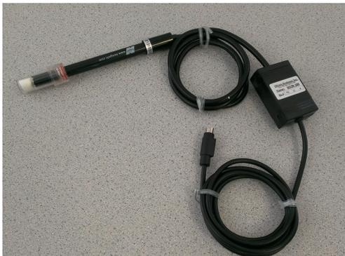
decreases as the concentration of oxygen in the polarograph chamber increases and decreases, respectively. The adapter then converts the changes in current to changes in voltage that can be recorded.
