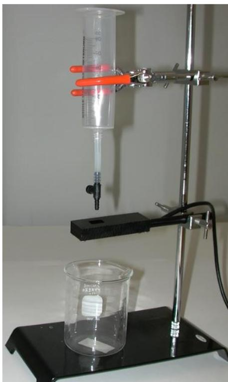
you see the signal on the waveform chart. A pulse will represent each drop.
