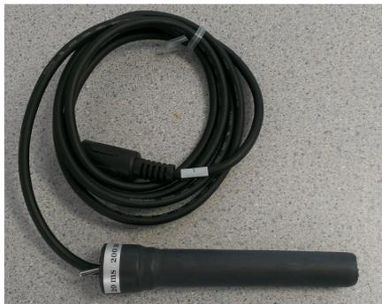
Conductivity is the ability of a substance to conduct an electric current. The principle by which conductivity is measured is fairly easy - two electrodes are placed in the solution, a potential is applied across the electrodes, and the current is measured. Conductivity (G) is the inverse of resistivity (R). This can be determined from the voltage and current values according to Ohm's law:
