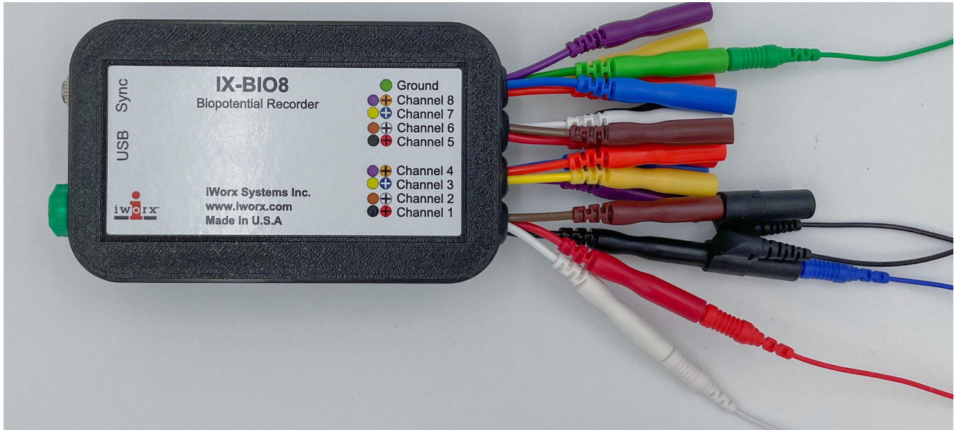
Figure 2: Six channel ECG connections on the IX-BIO8 recorder.
