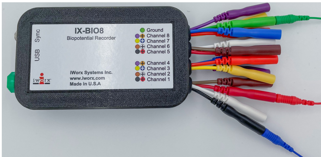
Figure 1: Single channel ECG connections on the IX-BIO8 recorder.
