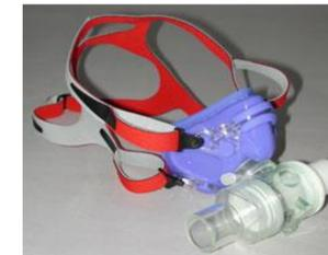
Figure 7. Face mask, head strap and valve for Iworx GA-300 gas analyzer.
