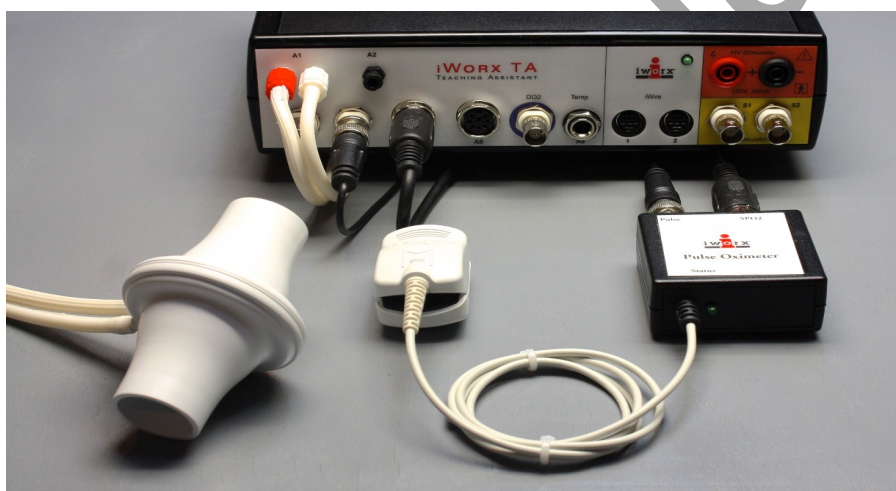
Figure HS-6-S3: A PO2-100D pulse oximeter and the flow head connected to the internal spirometer of the IXTA unit. NOTE – the iWire-PO2-100 will be plugged into the iWire 1 port on the front of the IXTA.
