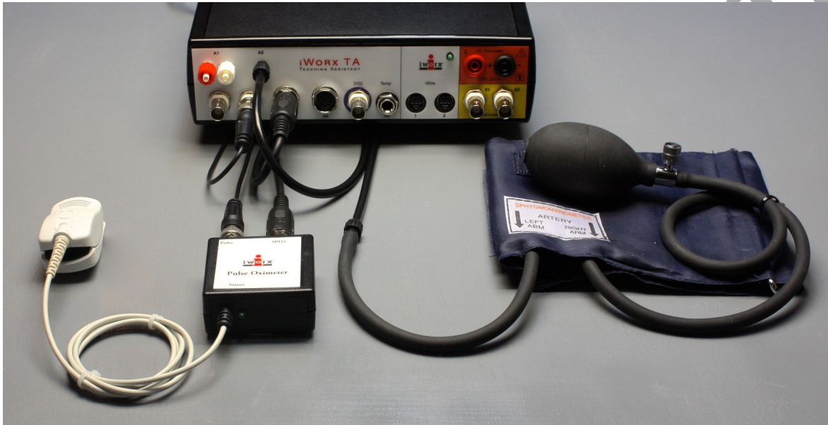
Figure HE-3-S3: The pulse oximeter and the BP-220 non-invasive blood pressure transducer connected to an IXTA. NOTE – the PO2 sensor will be plugged into the iWire port on the IXTA.
