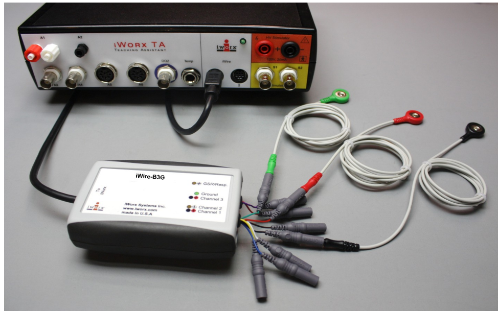
Figure HP-10-S2: The iWire-B3G cable connected to an IXTA.
