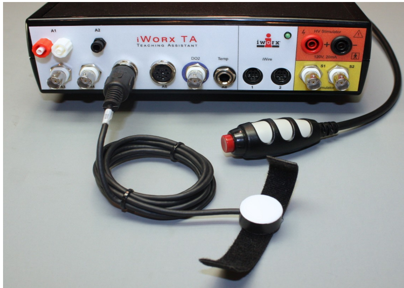
Figure HP-5-S3: The PT-104 pulse transducer and the EM-220 event marker connected to an IXTA.
