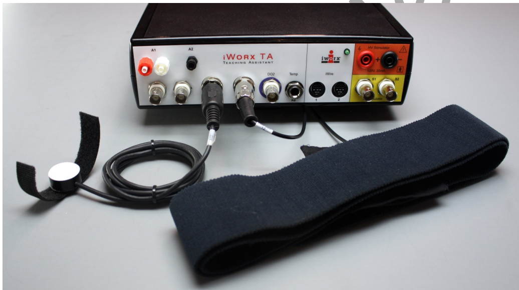
Figure HS-7-S3: A PT-104 pulse sensor and a RM-204 respiration monitor connected to an IXTA unit. The USB Pulse oximeter will connected directly to the computer via a USB port.
