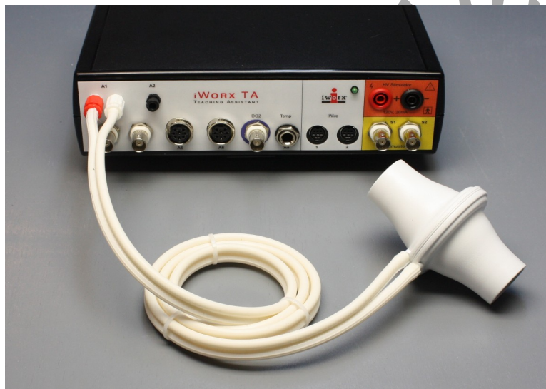
Figure HS-6-S3: The flow head connected to the internal spirometer of the IXTA unit. The USB Pulse oximeter will be connected directly to the computer.
