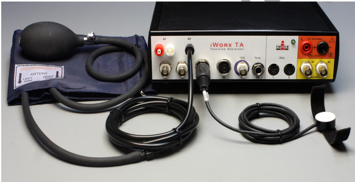
Figure HE-3-S3: The BP-220 non-invasive blood pressure transducer and pulse sensor connected to an IXTA. The pulse oximeter is connected via USB directly to the computer.
