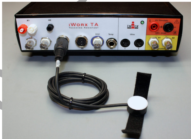
Figure T-T-S3: The PT-104 connected to the IXTA in the Tutorial experiment.
