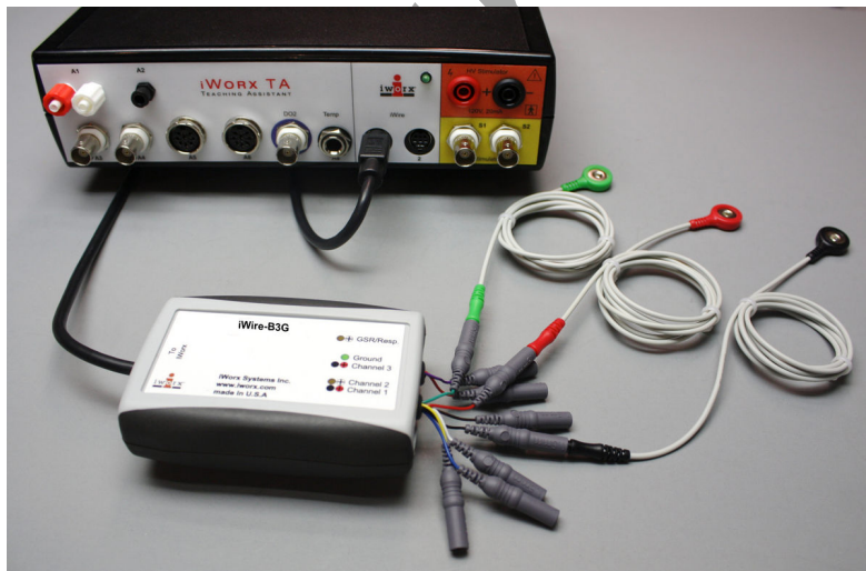
Figure T-T-S2: The iWire-B3G ECG cable with three lead wires attached connected to the IX-TA.
