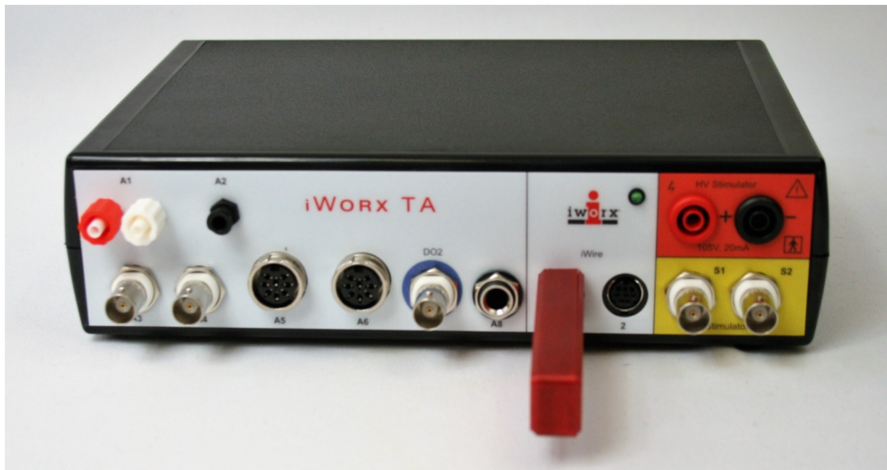
Figure HE-12-S2: The ROAM receiver connected to the IX-TA.
