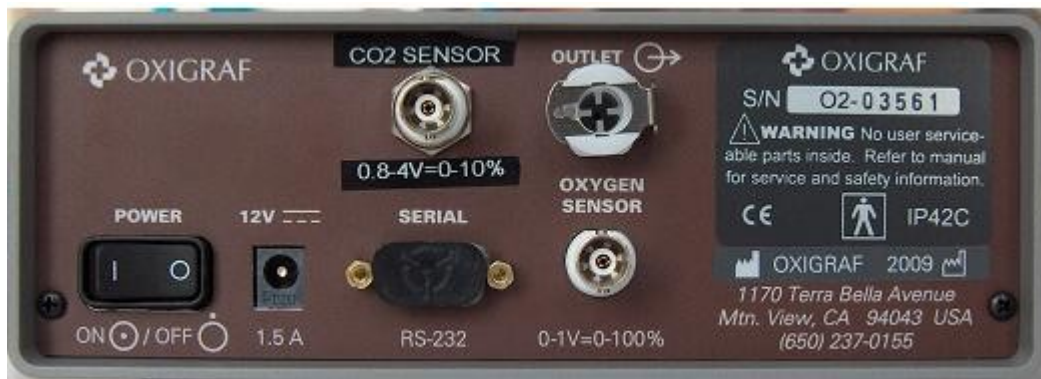
Figure AMe-1-S4: The rear panel of the GA-200B gas analyzer showing the outputs of the carbon dioxide sensor, on the left, and the oxygen sensor, on the right.
