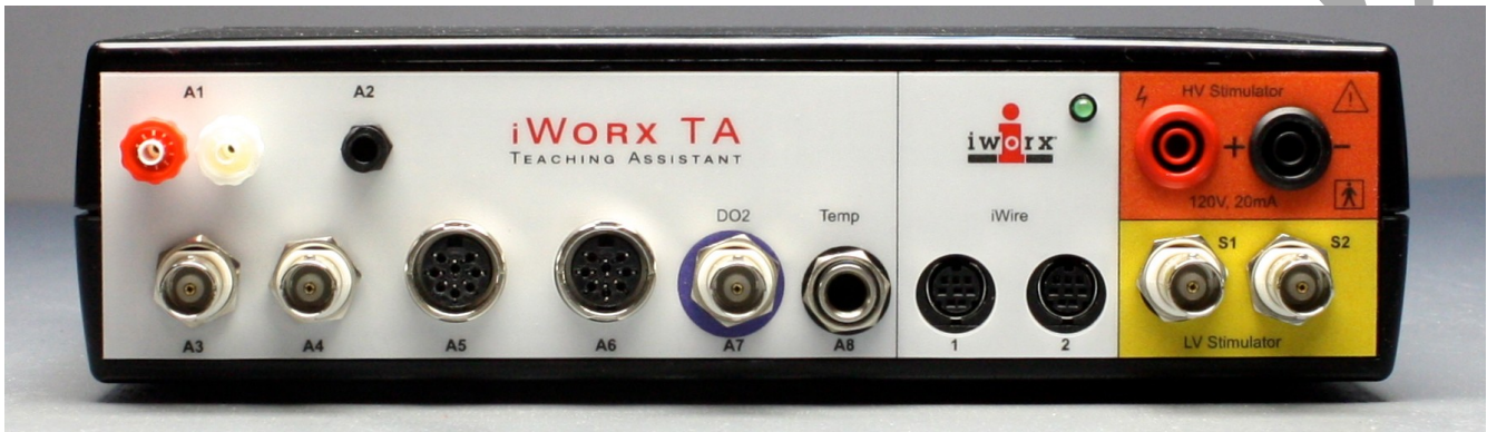
Figure AMe-1-S2: The front panel of the IXTA.
