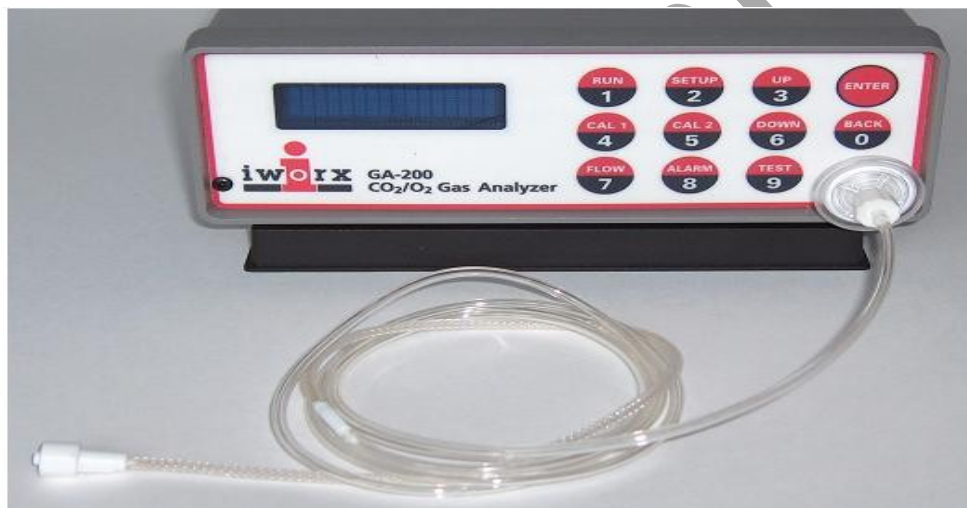
Figure AMe-1-S3: The GA-200 gas analyzer showing the proper connections of the Nafion tubing to the front filter to measure O_2 and CO_2 exchange.
