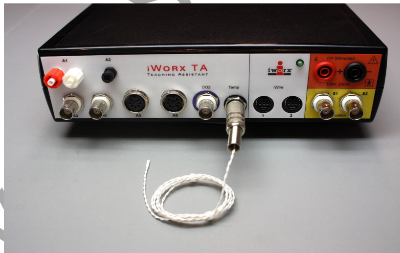
Figure HP-4-2: The TM-220 temperature probe connected to an IXTA.
