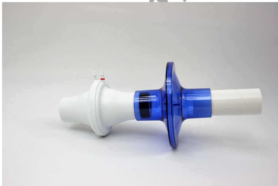
Figure HS-8-7: Full assembly of the flow head for the Restrictive portion of the lab.
