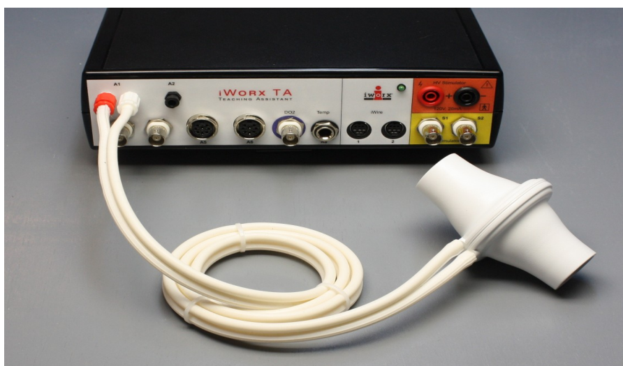
Figure HS-8-2: The flow head connected to the internal spirometer of the IXTA unit.
