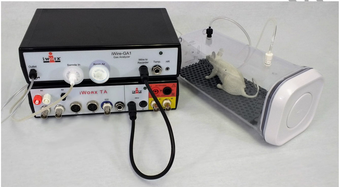
Figure AMe-1-S1: The front panel of both the IXTA and the iWire-GA showing the connections to and from the small animal chamber with the mouse inside.
