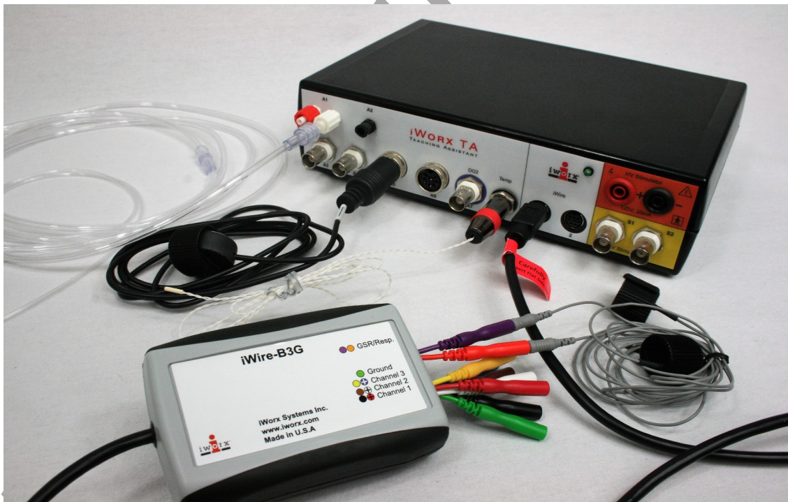
Figure HP-20-S1: The IXTA with the PT-104, the RM-220 plugged into the correct channels and showing the proper connection for the iWire-B3G GSR unit.
