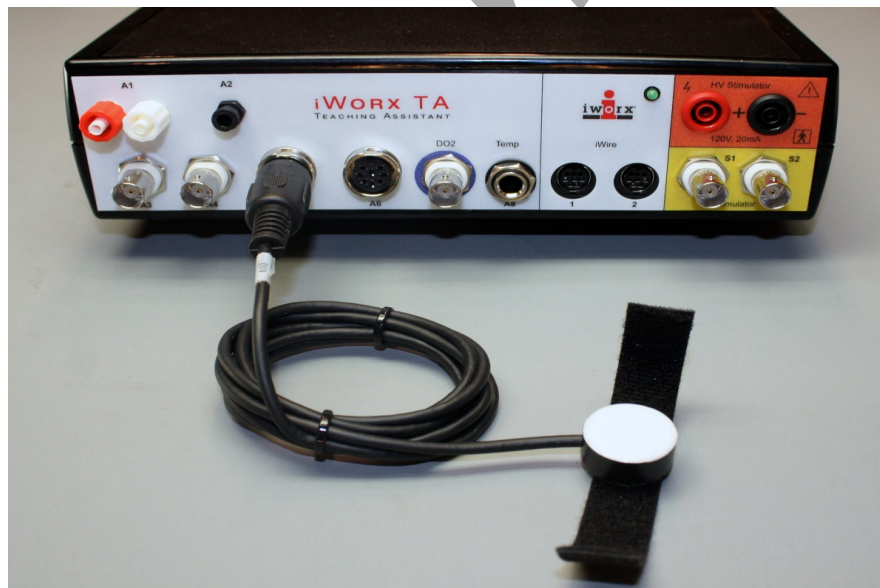
Figure HE-2-S1: The PT-104 pulse plethysmograph connected to an IXTA.
