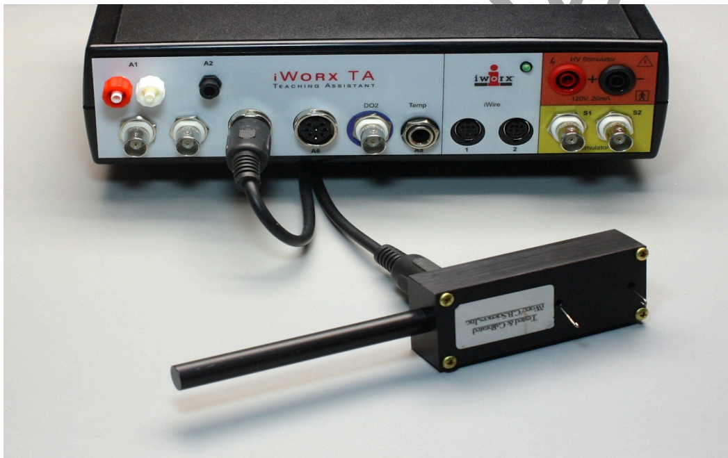
Figure AM-4-S5: The FT-302 dual-range force transducer connected to an IXTA.
