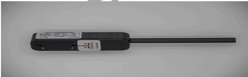
Figure AM-4-S3: The FT-302 dual-range force transducer.
