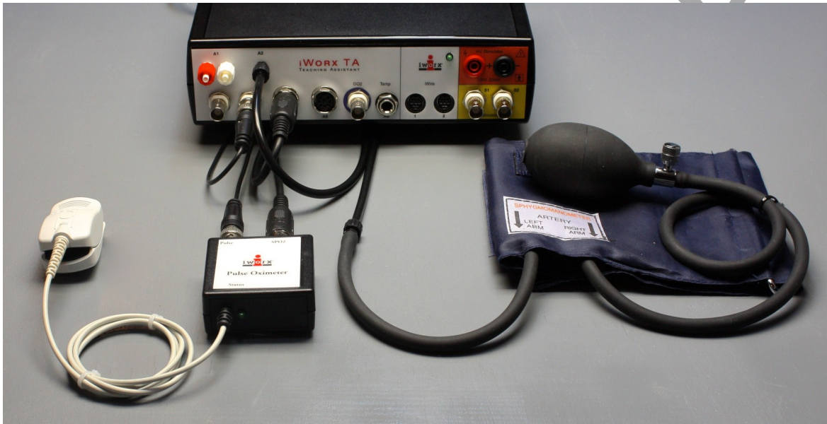
Figure HE-3-S3: The pulse oximeter and the BP-220 non-invasive blood pressure transducer connected to an IXTA.
