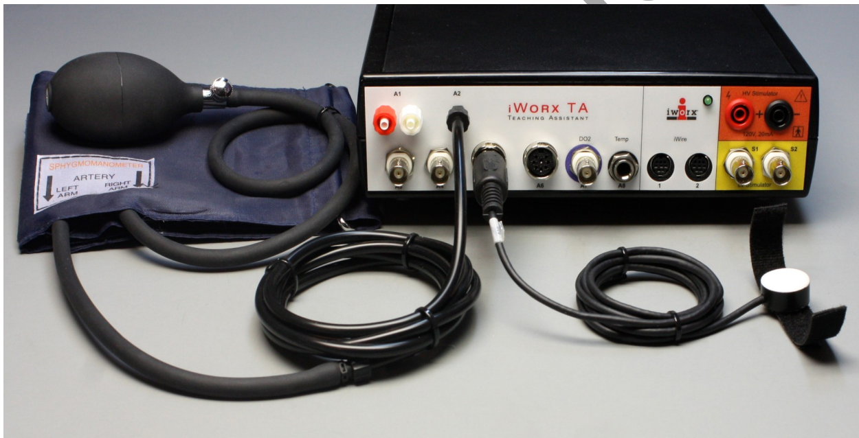
Figure HC-4-S3: The PT-104 pulse transducer and the BP-220 non-invasive blood pressure transducer connected to an IXTA.
