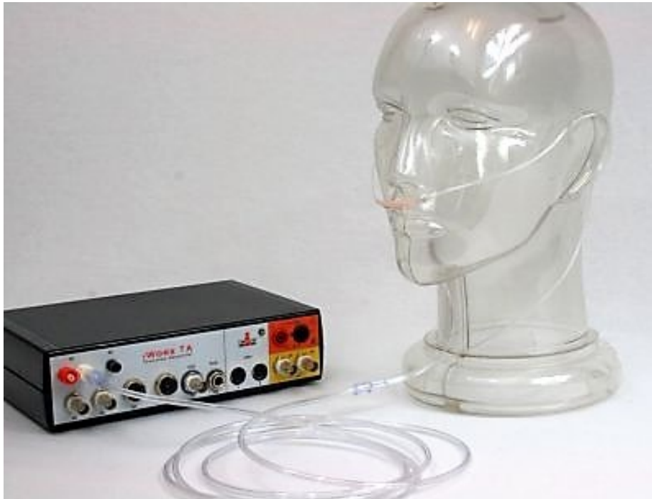
Figure HP-5-S2: Nasal cannula connected to the IX-TA and showing the proper positioning on the face.
