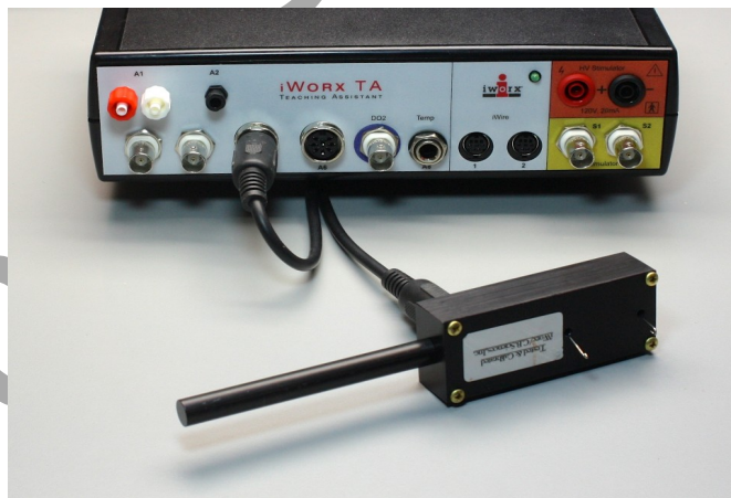
Figure FB-1-S2: The FT-302 force transducer connected to the IXTA.
