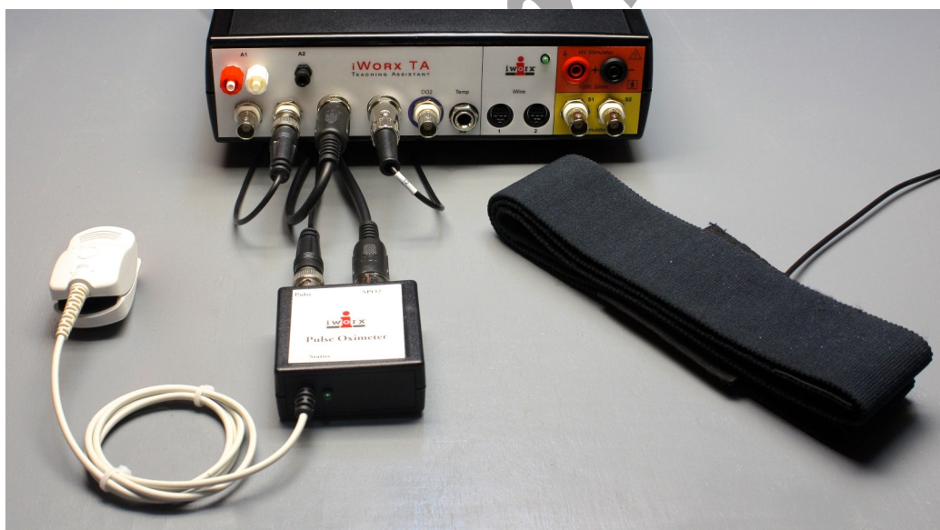
Figure HS-7-S3: A pulse oximeter and a RM-204 respiration monitor connected to an IXTA unit.
