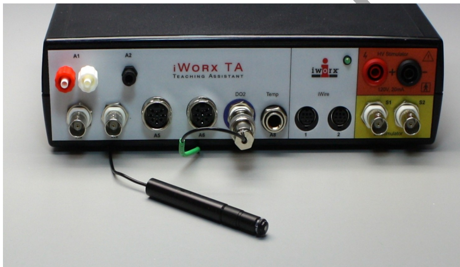
Figure CM-7-S3: Dissolved oxygen electrode (ISE-730) connected to an IXTA.
