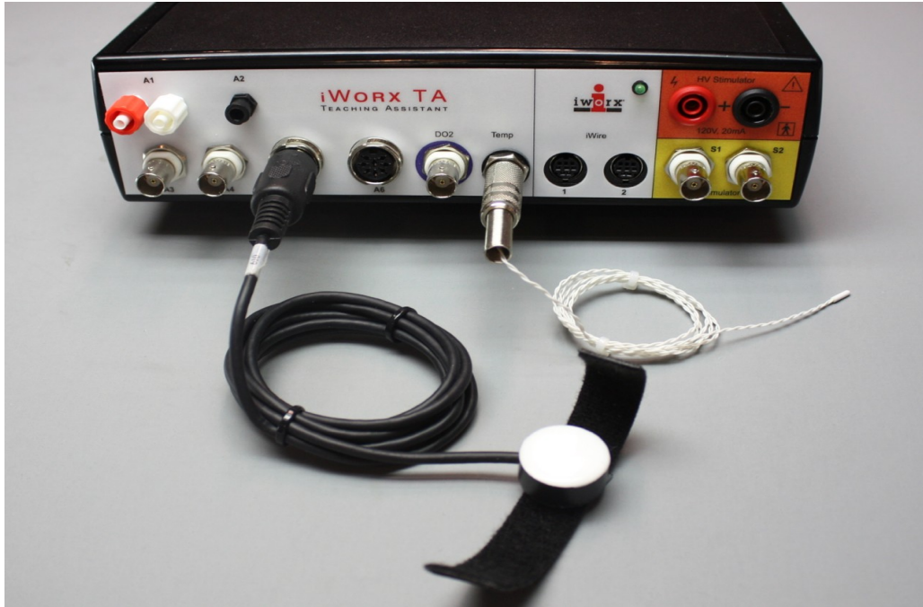
Figure HP-24-S7: The IXTA with the PT-104 and TM-220 plugged into the correct channels.
