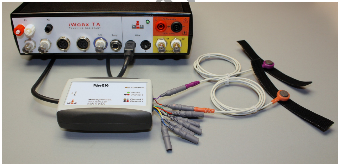
Figure HP-24-S2 The iWire-B3G ECG and Galvanic Skin Response amplifier. The purple and orange GSR electrodes are shown in this image.
