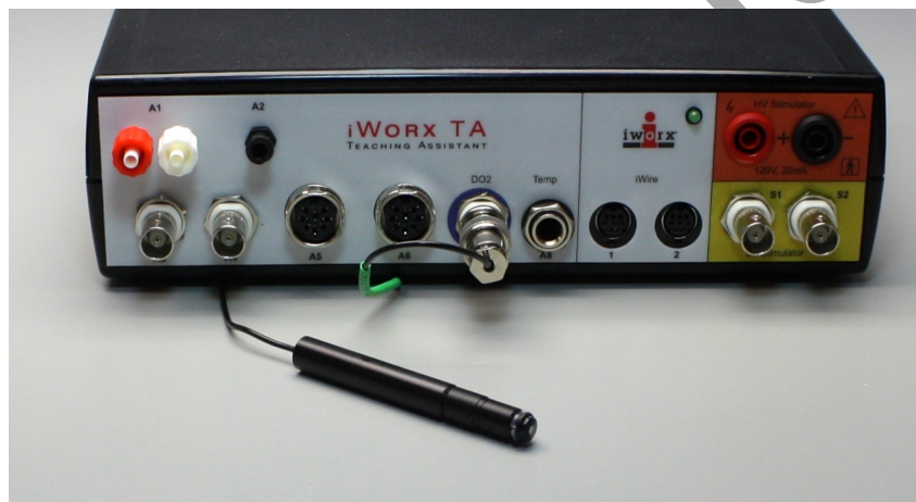
Figure CM-3-S3: Dissolved oxygen electrode (ISE-730) connected to an IWX-IXTA.
