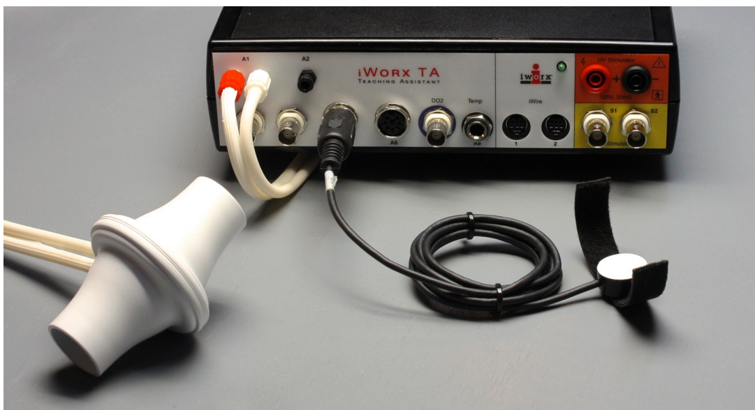
Figure HS-4-S3: A PT-104 pulse plethysmograph and the 300 L flow head connected to an IXTA unit.
