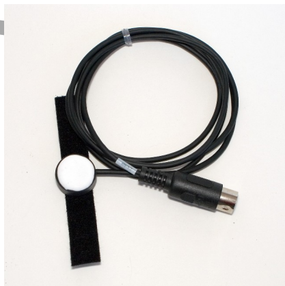
Figure HS-4-S2: The PT-104 pulse plethysmograph.
