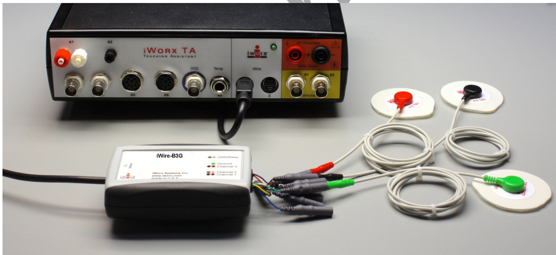
Figure HP-23-S3: iWire-B3G EOG cable attached to the front of the IX-TA.
