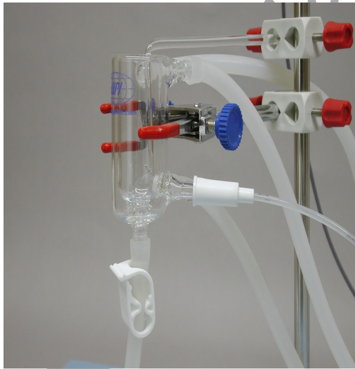
Figure AM-5-S7: 25 ml tissue bath in position for recording tissue tension.
