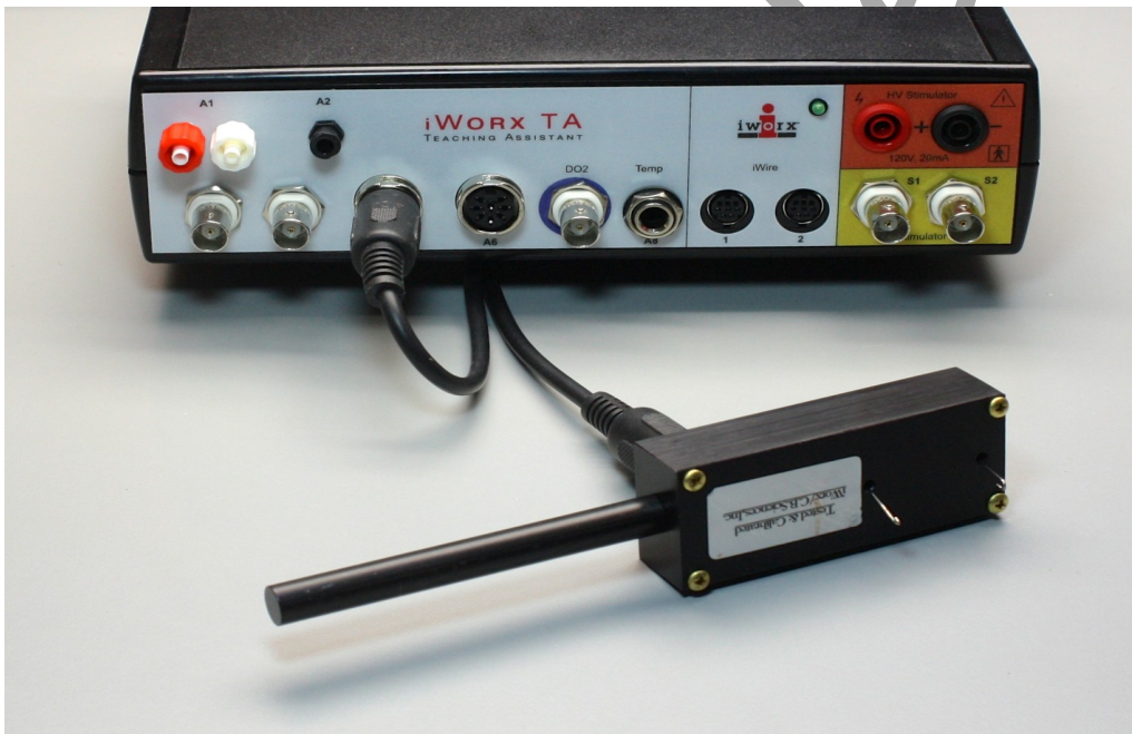
Figure AM-5-S5: The FT-302 dual-range force transducer connected to an IXTA with a male DIN-DIN cable.
