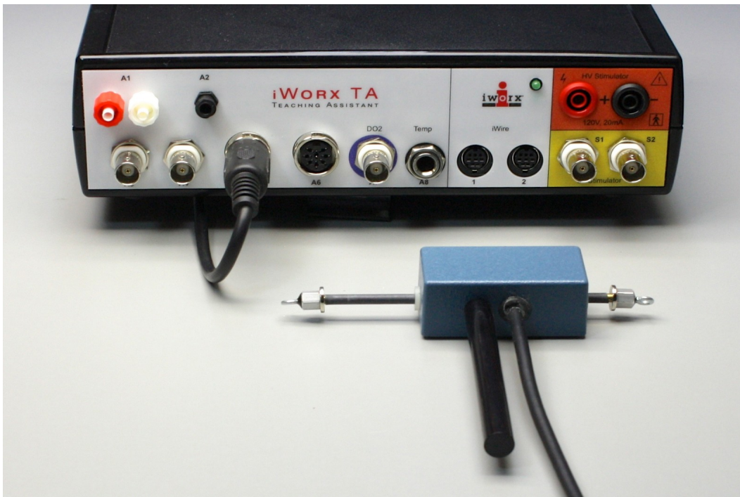
Figure AM-5-S2: The DT-475 displacement transducer connected to an IXTA.
