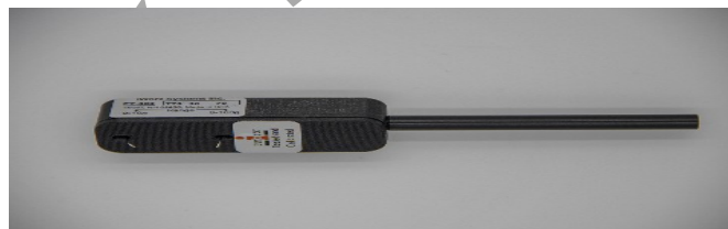
Figure AM-5-S3: The FT-302 dual-range force transducer.
