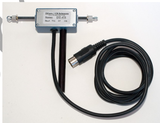
Figure AM-5-S1: The DT-475 displacement transducer.
