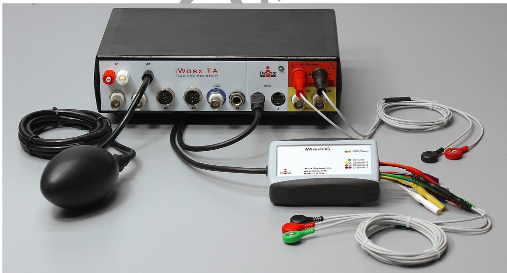
Figure HN-8-S1: IXTA with the FT-220, iWire-B3G and stimulator lead wires for performing the Human to Human Interface lab.
