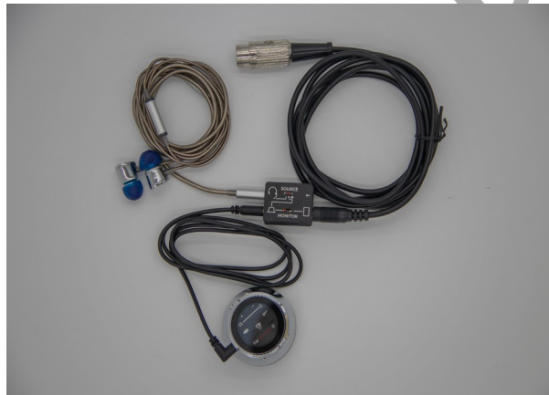
Figure HH-9-S1: The electronic stethoscope with Phono-DIN8 cable.
