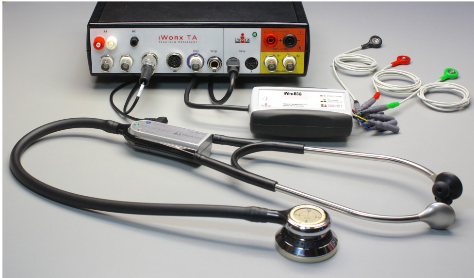
Figure HH-9-S2: The ECG cable and ES-300 electronic stethoscope connected to an IXTA.
