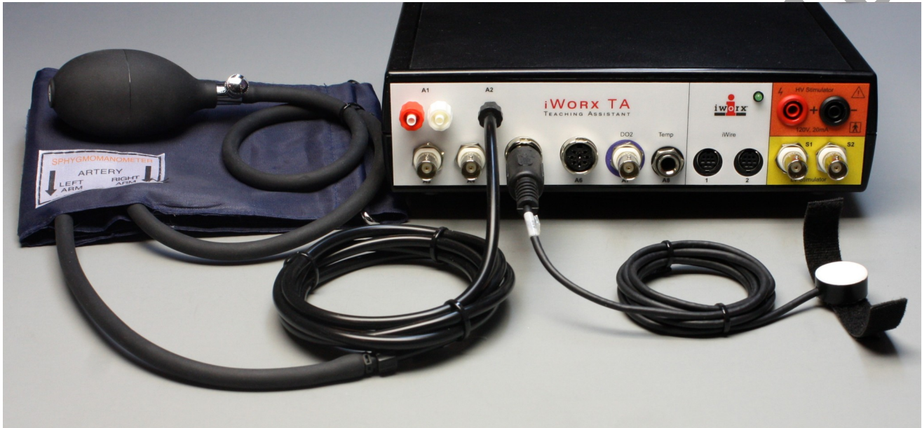
Figure HP-5-S2: The PT-104 pulse transducer and the BP-220 non-invasive blood pressure transducer connected to an IXTA.
