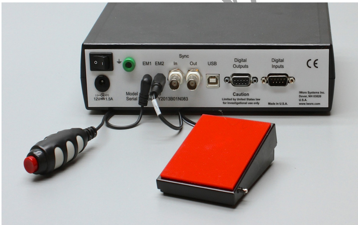
Figure HN-4-S2: The EM-220 event marker and FRS-220 connected to the EM ports on an IXTA.
