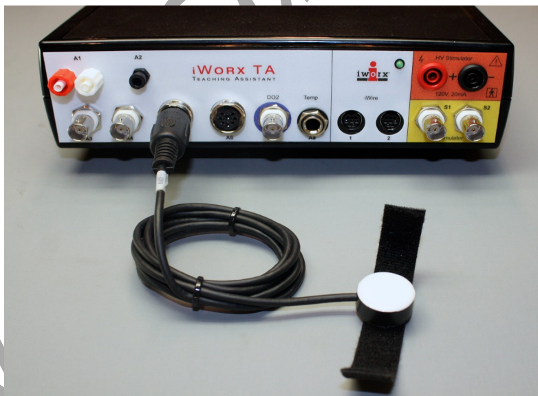
Figure HH-6-S1: The PT-104 pulse sensor connected to an IXTA.
