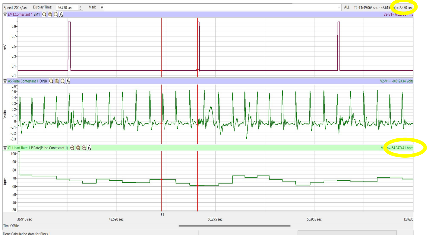
Figure HN-8-L3: A single trial for one question and answer by Contestant 1. The two cursors are positioned at the beginning of the F1 mark and on the leading edge of mark made by the event marker. Reaction time in this example is 2.450 sec and Mean HR is 65 bpm.
