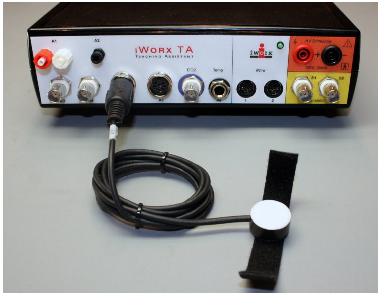
Figure HN-9-S3: IXTA with one PT-104 connected to channel A5. The 2 nd PT-104 will be connected to channel A6.
