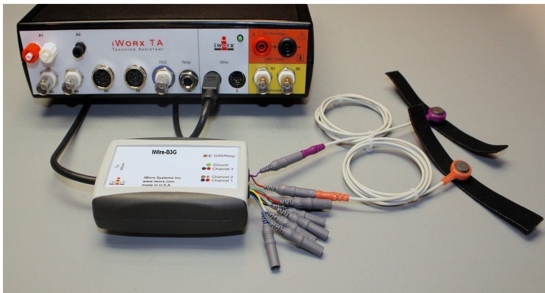
Figure HP-8-S2: The equipment needed to record GSR. The PT-104 plugs into Channel A5.
