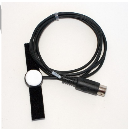
Figure HP-8-S1: PT-104 pulse plethysmograph.
