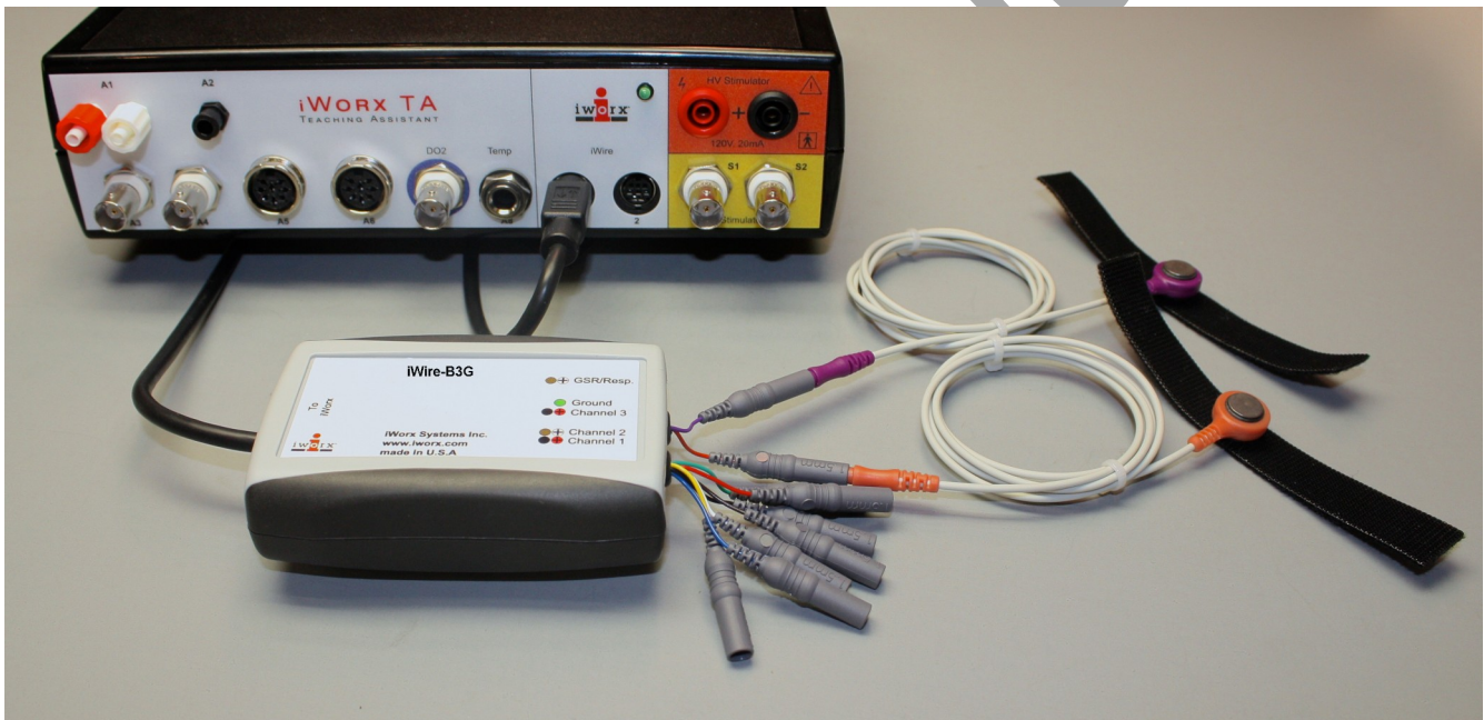
Figure HP-3-S1: The iWire-B3G galvanic skin response amplifier.
