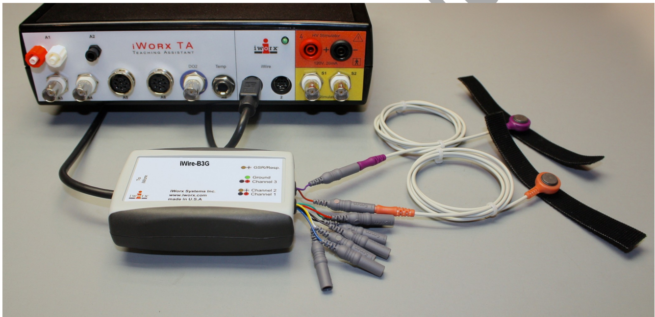
Figure HP-2-S1: The iWire-B3G galvanic skin response amplifier.
