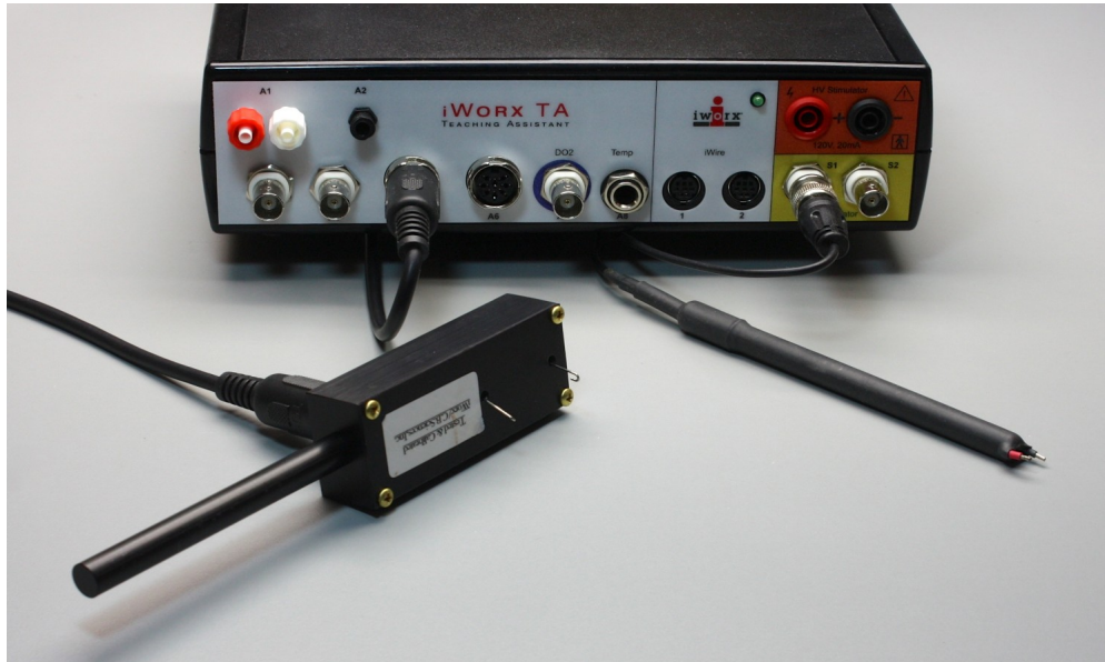
Figure AM-2-S3: The FT-302 force transducer and the A-BST-100 bipolar stimulating electrode connected to the IXTA.
