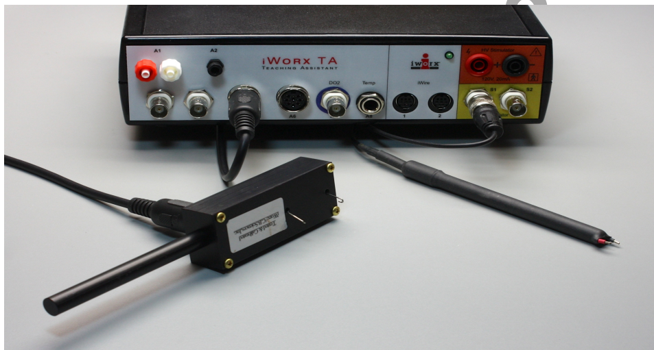
Figure AM-3-S3: The FT-302 force transducer and the A-BST-100 bipolar stimulating electrode connected to the IXTA.
