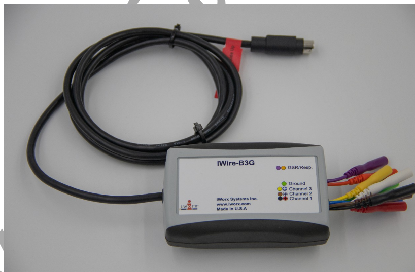
Figure AM-6-S1: The iWire-B3G ECG cable.
