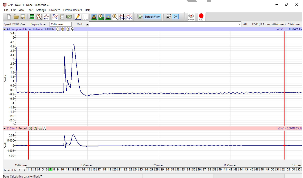
Figure AN-8-L6: Compound action potential (CAP) and stimulus pulse displayed in the Analysis window, with cursors positioned to measure the amplitude of the CAP.
