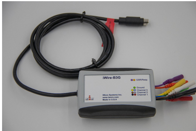
Figure AN-2-S4: The iWire-B3G recording cable.
