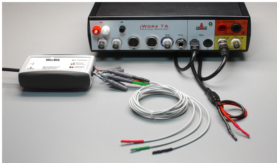
Figure AN-2-S5: The stimulator cable and iWire-B3G cable with three lead wires connected to the IXTA.
