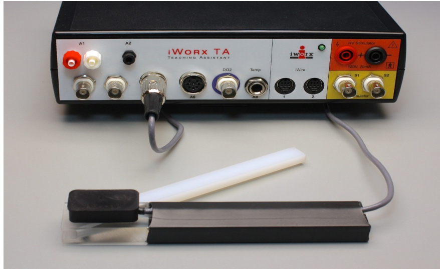
Figure HM-5-S2: The GN-100 goniometer connected to an IXTA.
