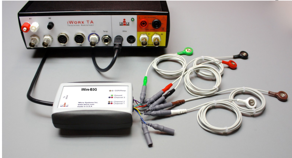
Figure HP-9-S1: The IXTA with the iWire-B3G and electrodes attached to the iWire input of the IXTA.
